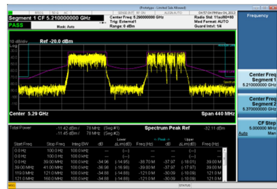
FIGURE 10. To conduct the 802.11ac spectral mask test on the channels in Figure 6, data is captured from 5090 to 5490 MHz.
