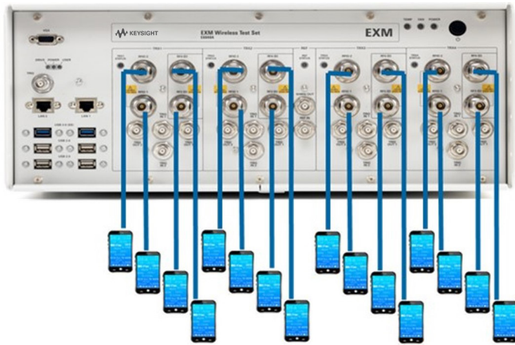
FIGURE 3. As shown here, the EXM permits the connection of up to 16 single-antenna DUTs.
